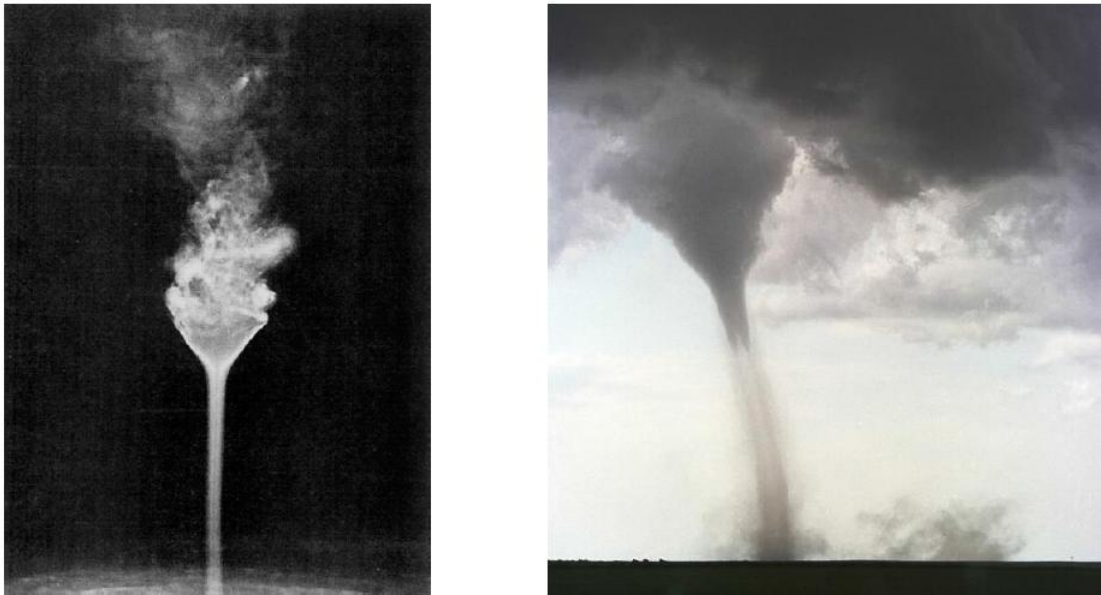
Fig. 2. Vortex breakdown in a vortex chamber [44] (left); vortex breakdown in a tornado [48] (right).
