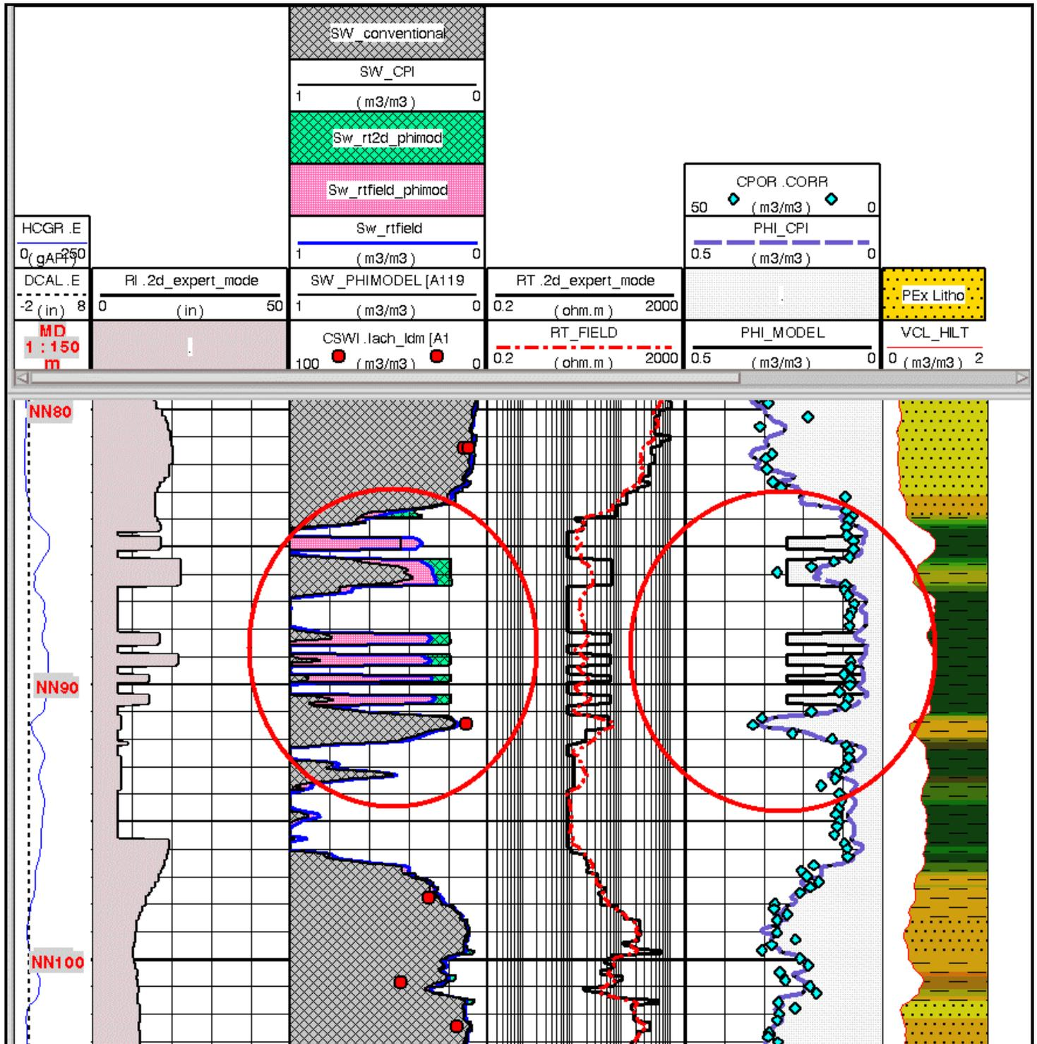
Fig. 8: Well 2. Comparison of water saturation profiles.
