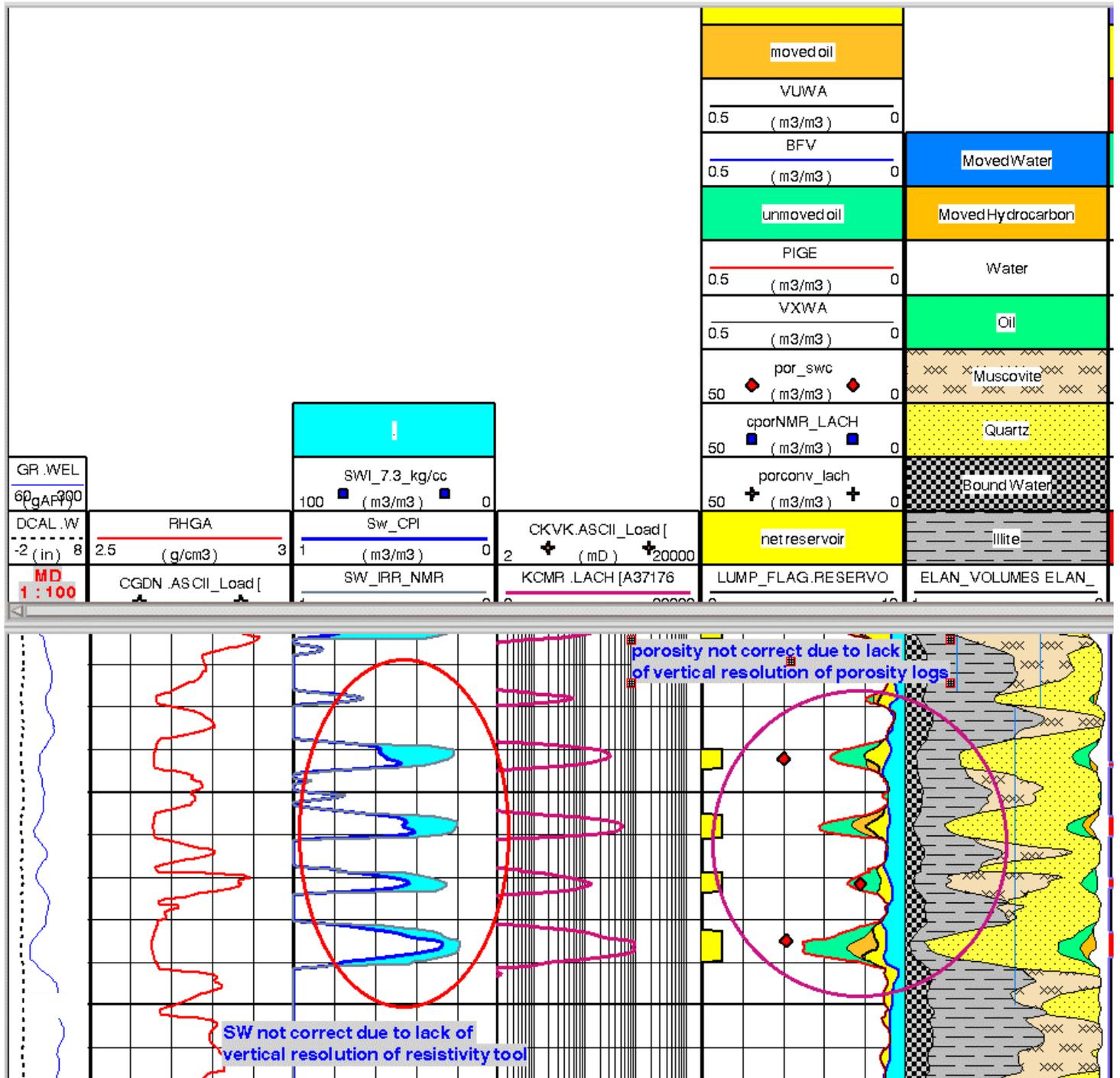
**Fig. 6: Well 1. Sequence of the thin beds: conventional interpretation.** This example from Well 1 shows a conventional interpretation of wireline logs (CPI). We can see that the estimated porosity is lower than core measurements (right dark-red oval) and that SW\_CPI is higher than SW\_IRR from NMR (left red oval).
