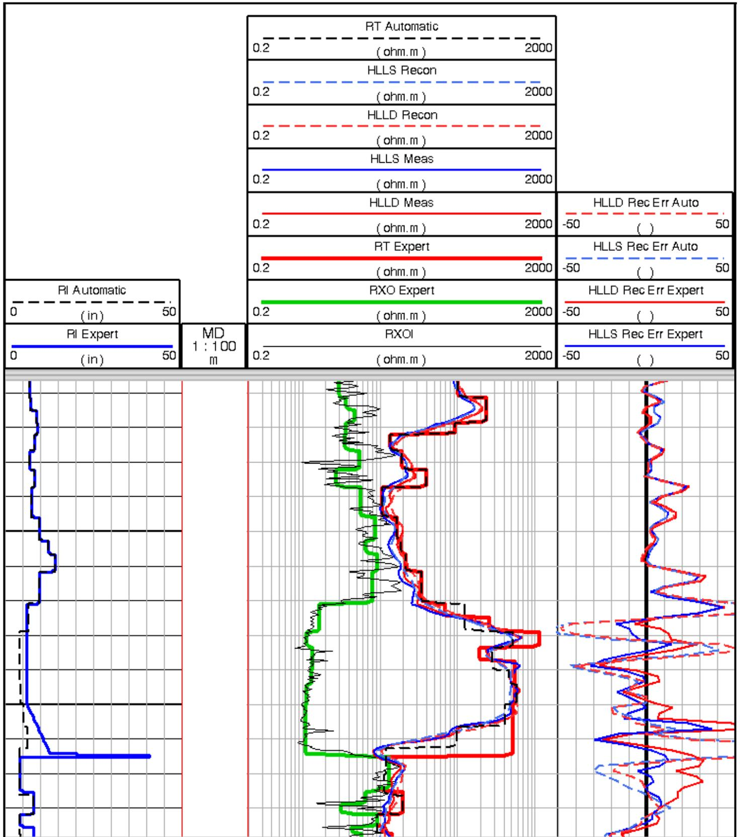
**Fig. 5: Well 1. Reconstruction of the anomalous invasion profile.** The invasion radius (left column, thick blue line) increases quickly at the bottom of the layer, thus triggering the anomalous Rt profile recorded by the resistivity tool (centre column, thin continuous lines). After the 2D expert-mode processing the final Rt profile (centre column, thick red line) is consistent along the whole layer.
