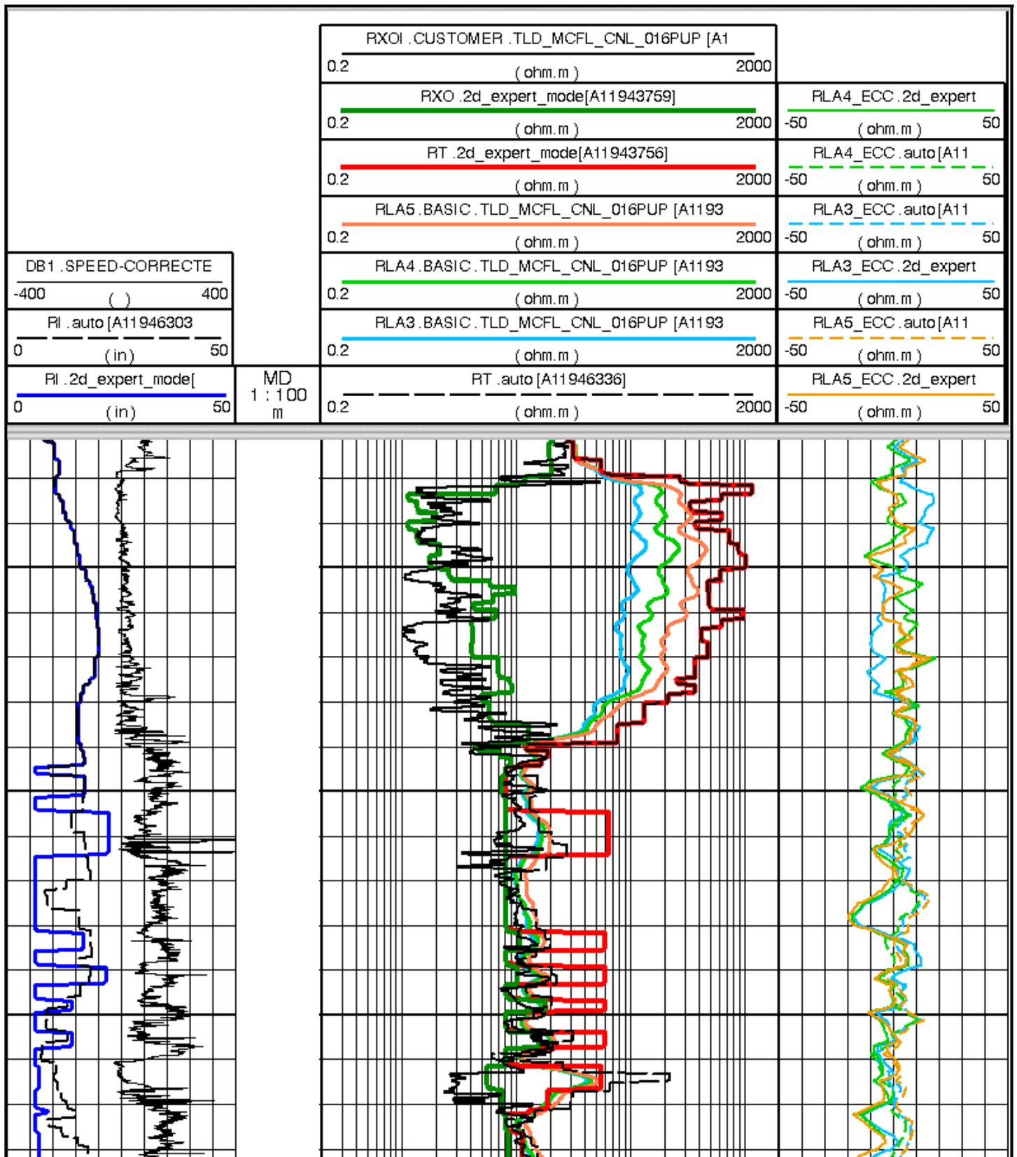
Fig. 7: Well 2. Sequence of thin beds: 2D modeling & inversion. The 2D automatic inversion computed a good log reconstruction (right column, dashed lines), but, due to the low sensitivity of the tool, didn't modify the very low resistivities in the thin beds (centre column, black dashed line). The 2D expert-mode processing did succeed in improving the  $R_t$  value in the thin layers (centre column, thick red line) while keeping the reconstruction errors very low.
