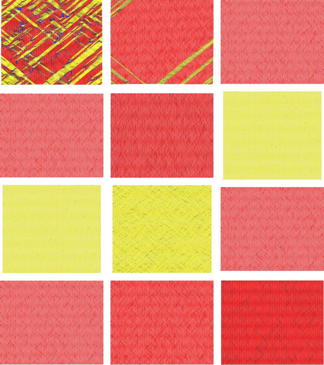
FIGURE 1. ( N = 100 ) First row: Uniaxial tensile loading \sigma_1 = 0.0, 0.15, 0.3 GPa with \sigma_2 = 0.0 GPa on the planes x_1 = -1/2 and x_1 = 1/2 after the first cooling. Second row: Biaxial loading \sigma_1 = 0.3, 0.15, 0.0 GPa for \sigma_1 + \sigma_2 = 0.3 GPa. Third row: Biaxial loading \sigma_1 = 0.0, 0.15, 0.3 GPa for \sigma_1 + \sigma_2 = 0.3 GPa. Fourth row: Uniaxial tensile unloading \sigma_1 = 0.3, 0.15, 0.0 GPa with \sigma_2 = 0.0 GPa.
